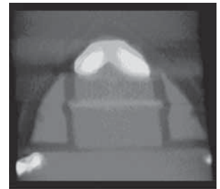
STEM tomogram of a memory cell obtained from a needle shaped FIB cut. Courtesy of H. Bender, imec, Belgium.
