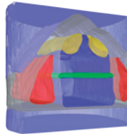
STEM tomogram of a memory cell obtained from a needle shaped FIB cut. Courtesy of H. Bender, imec, Belgium.
